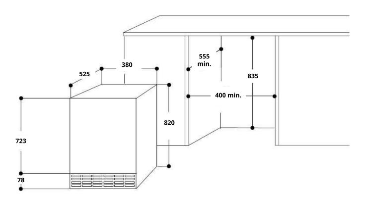
Measurements in millimeters.
