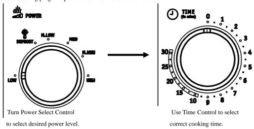
**NOTE:** As soon as the timer is turned, oven will start cooking. When selecting time for less than 2 minutes, turn timer past 2 minutes and then return to the correct time.
