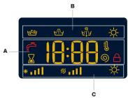
The duration of the available wash cycles and the remaining time of a running cycle appear in section A; if the DELAY TIMER option has been set, the countdown to the start of the selected wash cycle will appear. Moreover, pressing the relative button allows for visualising the maximum values for the temperature, spin speed or type of drying relative to the selected programme or the most recently selected ones, if compatible with the selected programme.
