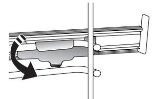
Please note: The sliding runners can be fitted on any level.
