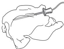
Insert the food probe deep into the meat, avoiding bones or fatty areas. For poultry, insert the probe lengthways into the centre of the breast, avoiding hollow areas. Place the food in the oven and connect the plug by inserting it into the connection provided on the righthand side of the oven's cooking compartment.
