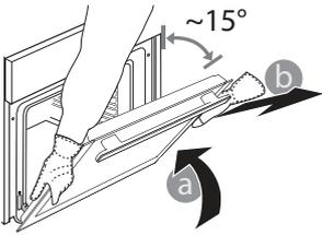
3. Refit the door by moving it towards the oven, aligning the hooks of the hinges with their seating and securing the upper part onto its seating.
