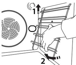
2. Pull the heating element out a little and lower it.
