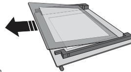
To correctly reposition the inner glass, make sure that the "R" is visible in the left-hand corner and the clear surface (not printed) is facing up. First insert the long side of the glass indicated by "R" into the support seats, then lower it into position (4). Refit the upper edge (5): a click will indicate correct positioning. Make sure the seal is secure before refitting the door.
