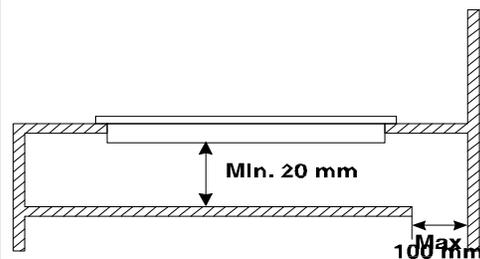
The diagrams illustrate the cutting sizes and additional shaping required for the installation hole if you decide to install the hob flush with the work-top surface. The work-top hole and shaping dimensions are purely guideline; it is essential to refer to your actual ceramic hob before making any cuts.
