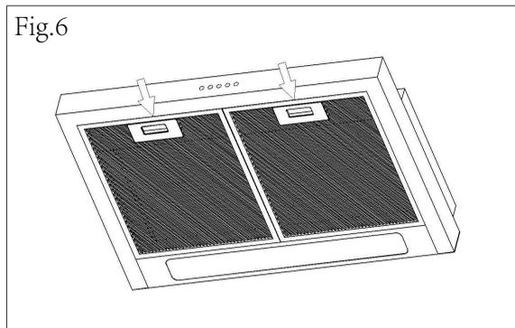
The active carbon filters purify the air that is replaced in the environment. The filters are not washable nor reusable and must be replaced every 4 months at most. The saturation of the active carbon filter depends on the frequency of use of the appliance, the type of cooking and the regularity of cleaning the aluminum filters.
