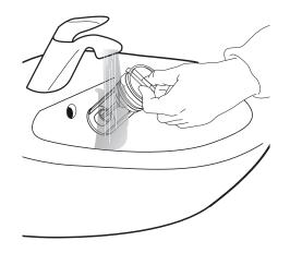
**6.** Insert the water filter and reinstall the kick panel: Re-insert the water filter by turning it clockwise. Turn it as far as it will go; the filter's grip should be in its vertical position. In order to check the filter's seal, pour about 1 litre of water into the detergent dispenser. Re-install the kick panel.
