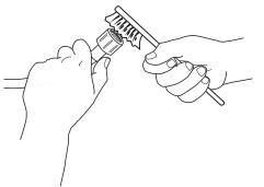
**3.** At this point, manually unscrew the intake hose from the back of the washer dryer. Using pliers, extract the mesh filter from the valve on the back of the washer dryer and clean it.
