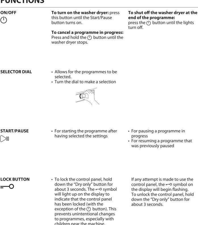
If any attempt is made to use the control panel, the -- o symbol on the display will begin flashing. To unlock the control panel, hold down the "Dry only" button for about 3 seconds.
