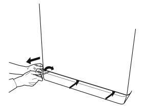
**2.** Container for the drained water: Place a low and wide container under the water filter in order to collect the residual water.
