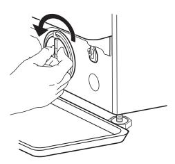
**4**. Remove the filter: Place a cotton cloth under the water filter in order to absorb any small amounts of residual water. Next, remove the water filter by turning it counter-clockwise.
