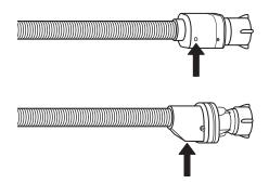
For flood protection hoses: check the safety valve's inspection window (see the arrow). If it's red, this means that the flood protection function has been engaged; in this case, the hose will have to be replaced with a new one. In order to detach the hose, press the release button (if present) and unscrew the hose.
