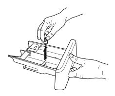
**3.** Wash the components under running water, taking care to remove all the detergent and fabric softener residues.
