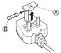
Remove the fuse cover (A) and the fuse (B).
