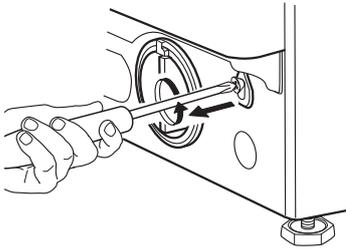
**4.** Afterwards, reattach the cord by inserting the screw with the help of a screwdriver.
