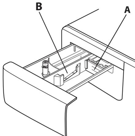
Preferably use the partition **A** when washing with a liquid detergent for washing, to ensure that the correct quantity of detergent is used (the partition is included in the bag containing the instructions).
