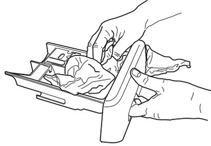
**2.** Remove the insert from the fabric softener compartment.
