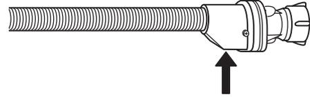
For flood protection hoses: check the safety valve's inspection window (see the arrow). If it's red, this means that the flood protection function has been engaged; in this case, the hose will have to be replaced with a new one. In order to detach the hose, press the release button (if present) and unscrew the hose.
