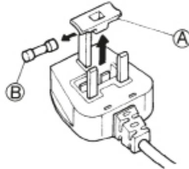
1. Remove the fuse cover (A) and the fuse (B).
