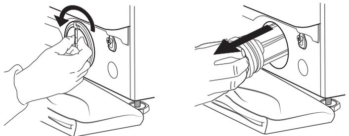
**5.** Clean the water filter: remove any residues from the filter and wash it under running water.
