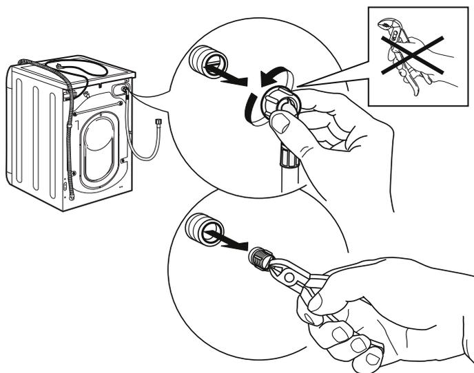
**4.** Re-insert the mesh filter. Reconnect the intake hose to the water tap and the washer dryer. Do not use tools to connect the intake hose. Open the water tap and check to make sure that all the connections have been tightened properly.
