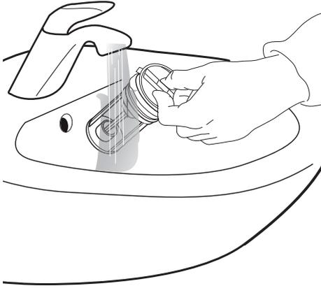
**6.** Insert the water filter and reinstall the kick panel: Re-insert the water filter by turning it clockwise. Turn it as far as it will go; the filter's grip should be in its vertical position. In order to check the filter's seal, pour about 1 litre of water into the detergent dispenser. Re-install the kick panel.
