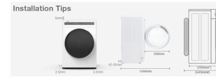
Product Depth\* : include door and button Product Depth<sup>#</sup> : include door, button and hose at back Dimensions listed are for references only.
